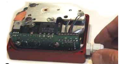
6.- Hand tighten the liquid tight fitting to establish seal
