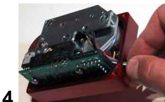
4.- Insert the cable into the actuator base
