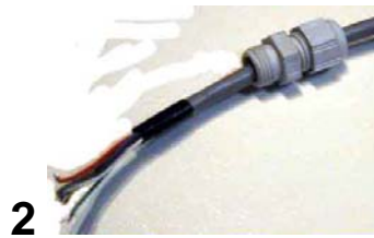
2.- The cable has to be stripped of its jacket for 2 inches (50mm) and the wires need 1/8" (3mm) stripped ends
