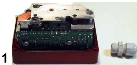
1.- Remove the liquid tight fitting from the actuator casing and insert the cable into it.
