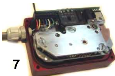
4.- Insert the cable into the actuator base
